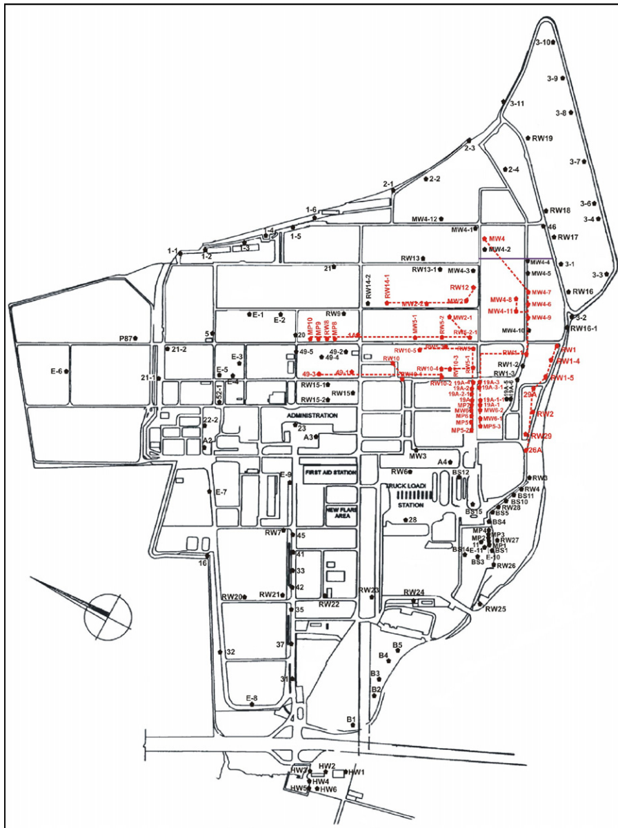
Fig. 5. Bioslurping wells network within the facilities of the refinery.
